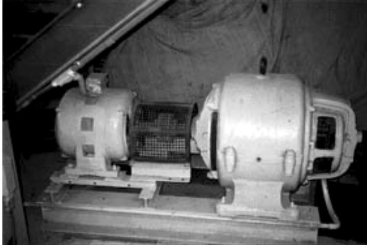
15 HP motor generator now used as a test set
