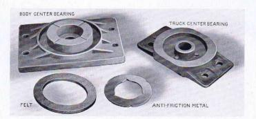
HE difference between the old-fashioned center bearing and the Brill Oil-Retaining Center Bearing is simply an allowance of space in the latter for an oil reservoir, and there is also a phosphor bronze ring to take the wear and a felt ring to exclude dust. But slight as these changes are, they make all the difference between a grease center bearing and one lubricated with oil. Grease is not a satisfactory
