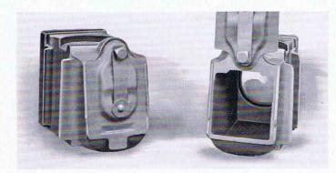
HEN used with truck No. 27-M. C. B. the top of the box is made with pockets in which the ends of the equalizers rest; otherwise it is the same as shown in the illustration.
