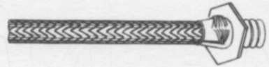
Fig 5 Wires bent close to Ter- minal (on one side) ready for soldering.
