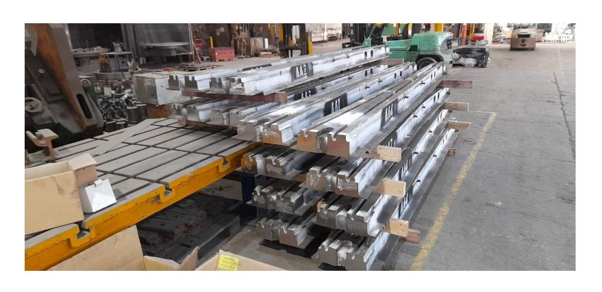
Six sets of new point and crossings cast by Beckwith Iron and Steel Co. of Melbourne with point mechanisms from Hanning Kahl of Germany were acquired.
