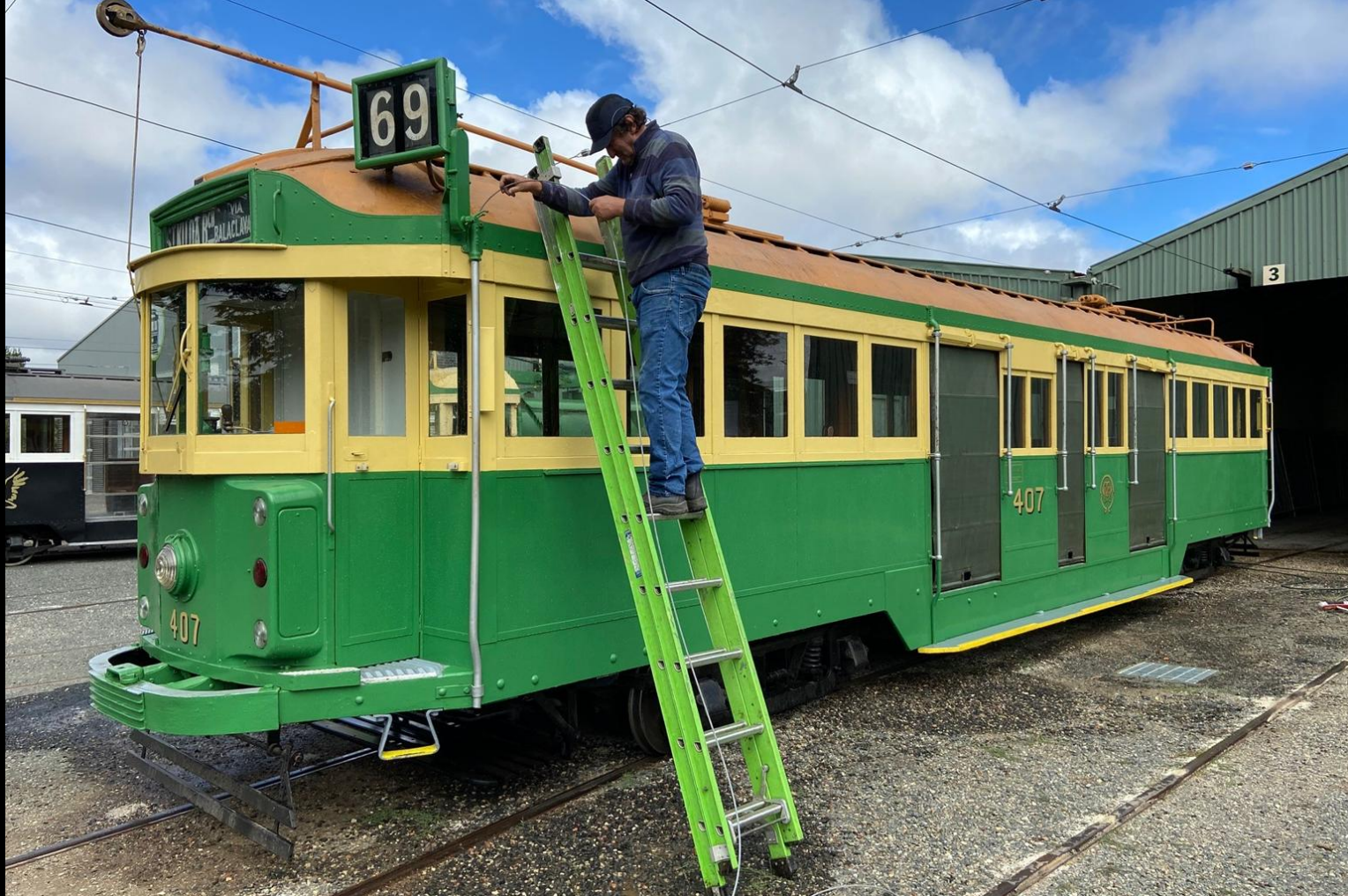
Tony clearing debris from the roof drain on W2 407
