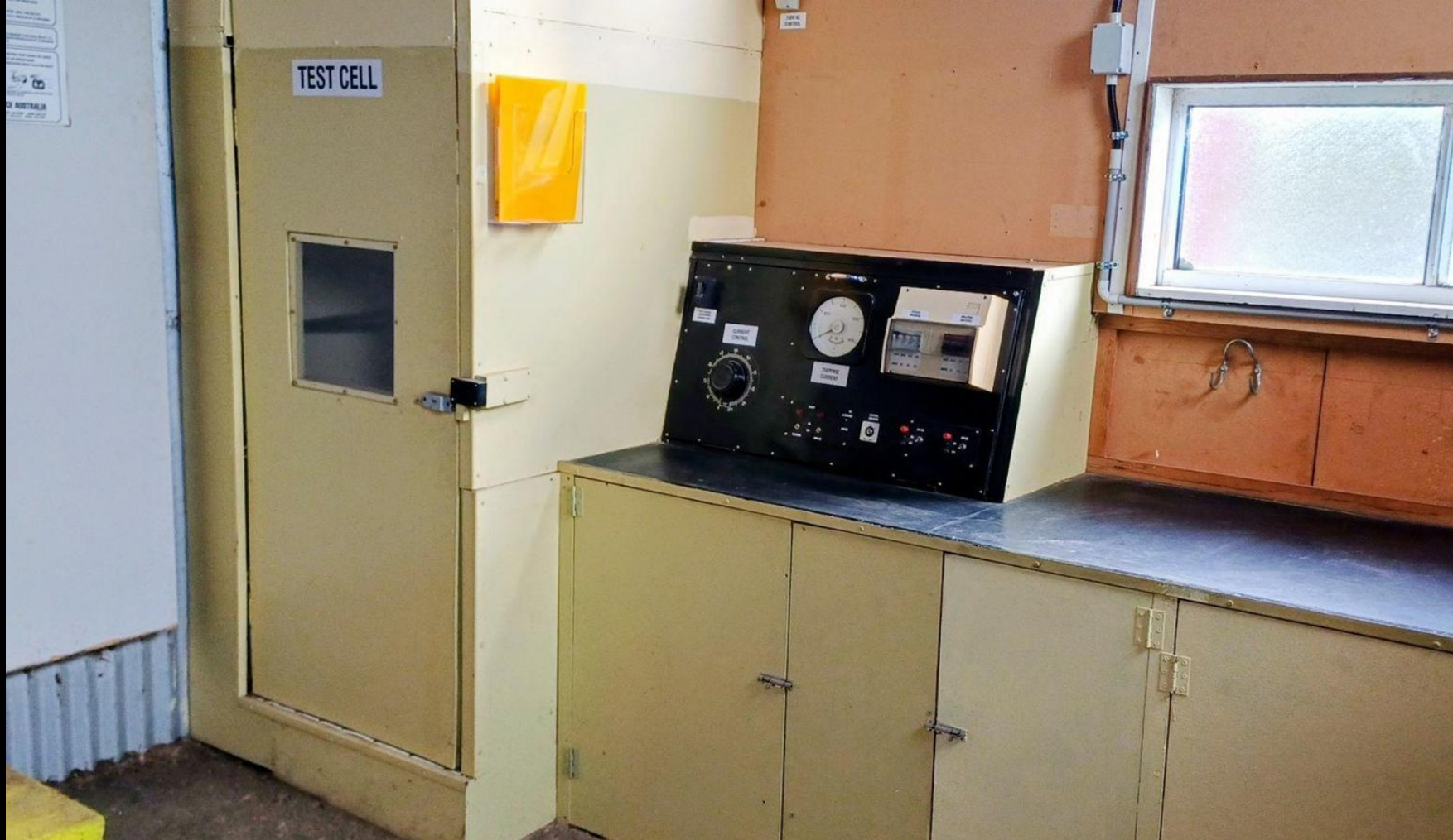
Test bench for electrical switches, line breakers and coils
