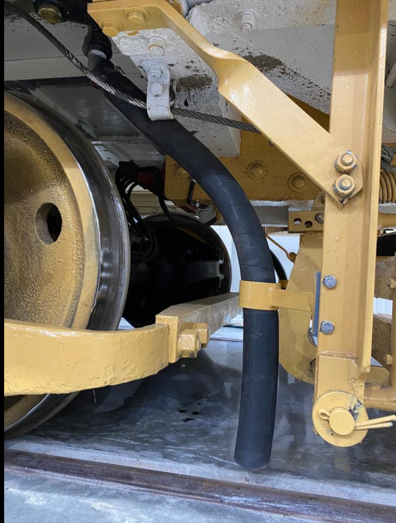
Greasing axle boxes and installing new sand pipes on VR 41
