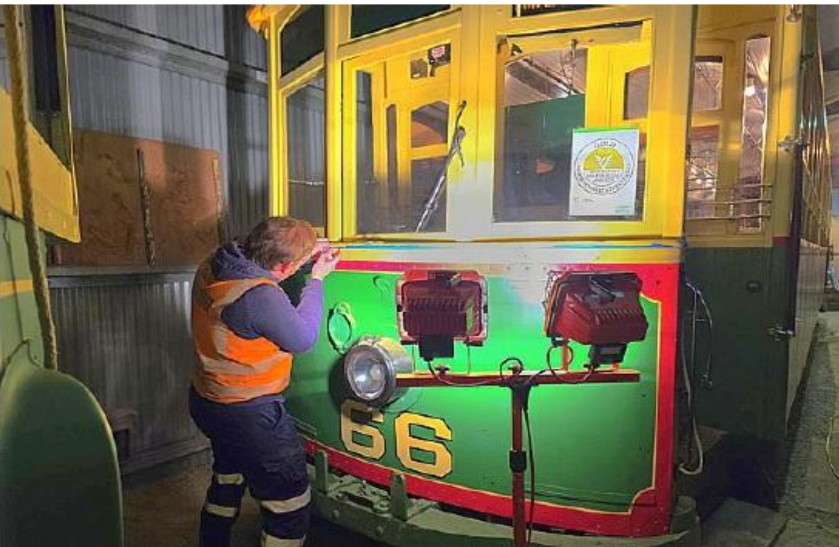
Shane Parsons applying tape in preparation for corrective painting on Perth E 66. 2 August 2024. Photograph: Daniel South
