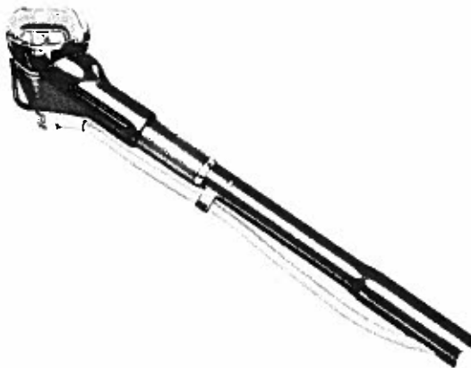
Assembly of Type G Collector on End of Trolley Pole
